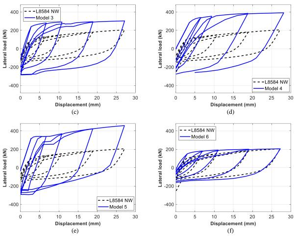
Figure 4. (a-f) Load-deflection behavior of model 1-6
