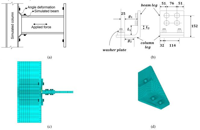
Figure 1. (a) experimental specimen, (b) geometric details of angle, (c) FE model, and (d) FE model of stiffened angle.
