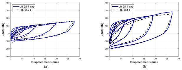
Figure 2. Comparison of the load-deformation behavior between experimental and FE model: (a) L8-58-7, and (b) L8-58-
