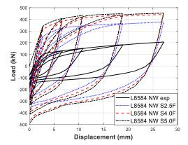
Figure 3. Effect of stiffener thickness on load-displacement behavior
